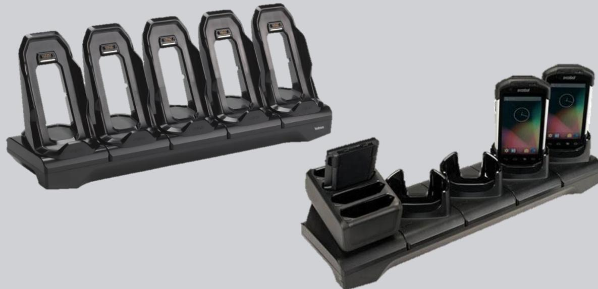
The 5-Slot ShareCradles provide high density & flexibility. Available in charge-Only or Ethernet variants, the 5-Slot Share Cradles can accommodate either 5x or 4x TC70(x)/TC75(x) Series plus 4x spare batteries off of one power supply via the 4-Slot Battery Charger Adapter Cup (*Sold Separately*). The 5-Slot ShareCradles can be racked/mounted in a standard 19 in. rack system via the mounting accessory.
